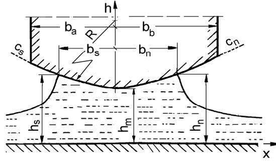
Fig. 3. Sketch of a barrel piston ring
