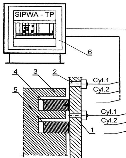
Fig. 1. Schematic of the SIPWA-TP diagnostic system; 1 – inductive sensor, 2 – temperature sensor, 3 – piston, 4 – SIPWA system ring, 5 – second piston ring, 6 – monitoring set [4]
