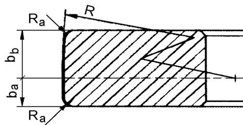
Fig. 9. Schematic of the RT marine engine piston ring
