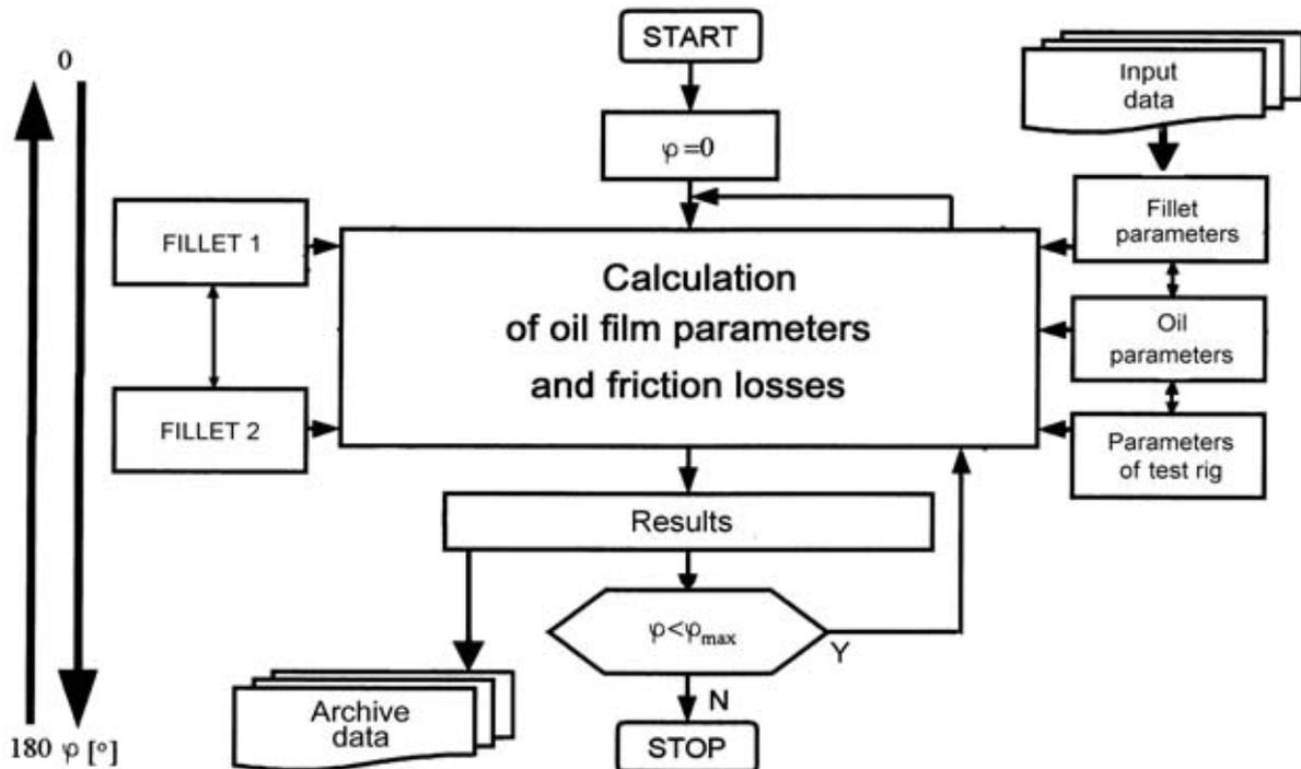
Fig. 2. The flow chart of test stand mathematical model [3]
