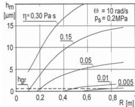
Fig. 8. Changes in minimum oil film thickness  $h_m$  vs. profile curvature radius  $R$ , for different oil viscosities
