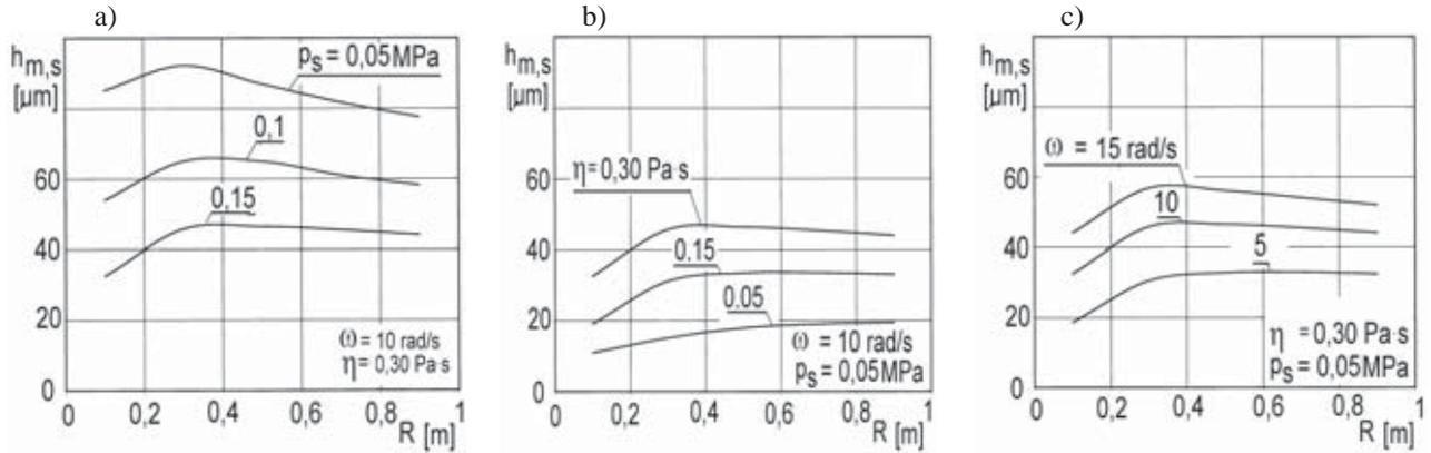
Fig. 6. Changes in the  $h_{m,s}$  mean minimum oil film thickness vs. the  $R$  ring profile curvature radius for selected values of ring operation parameters (values shown in charts)
