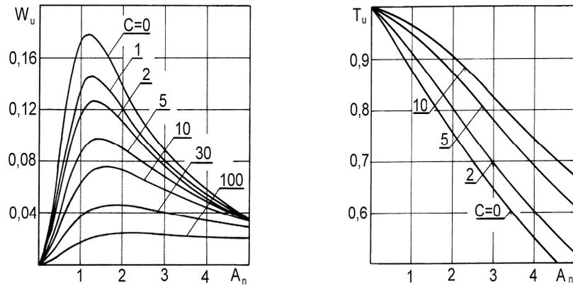
Fig. 4. Course of the  $W_u$  and  $T_u$  factor vs. the  $A_n$  coefficient for selected values of the  $C$  factor characteristic for double barrel ring
