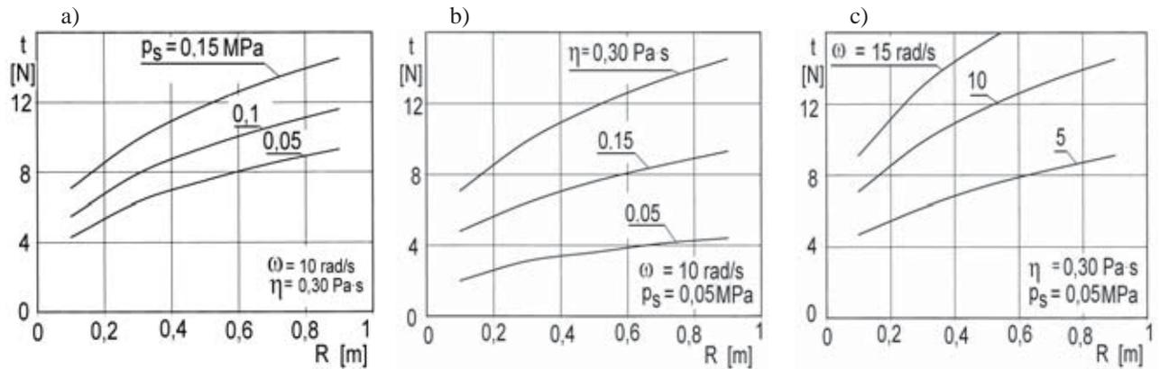
Fig. 7. Changes in the  $t$  mean friction force vs.  $R$  ring profile radius for selected values of ring operation parameters (given in Figs.)
