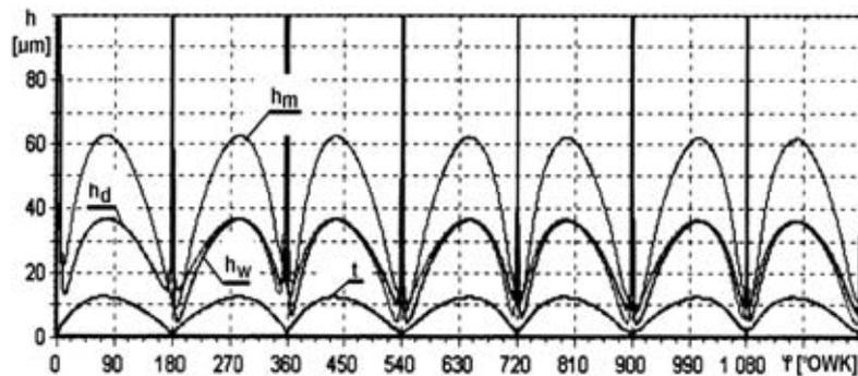
Fig. 5. Exemplary courses of the oil film minimal value ( $h_m$ ), oil layer thickness before ( $h_d$ ) and behind ( $h_w$ ) the ring and friction force vs. crank angle
